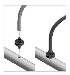
• PCJ with Press-Fit connector and straight Press-Fit to barb adaptor
