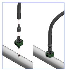
• PCJ with Press-Fit connector and elbow Press-Fit to barb adaptor
