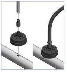
PC with Press-Fit connector and elbow Press-Fit to barb adaptor
